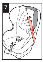
From the front, pull pad off the shell, starting at the top. Lift pad over the harness strap holders and work the pad around the harness adjustment cover.
